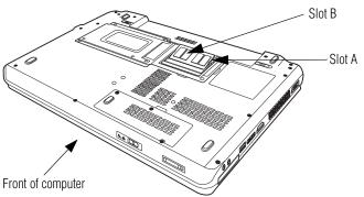
(Sample Illustration) Removing the memory module
